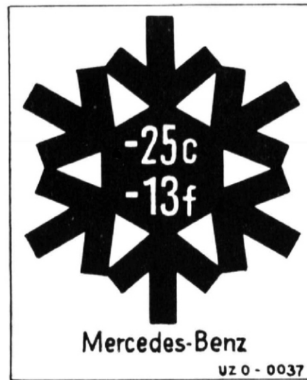
Figure 31 Antifreeze filling to -25^{\circ}\text{C} or -13^{\circ}\text{F}
