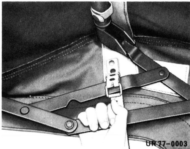
Figure 110 Pull folding top scissors downward 404.1
