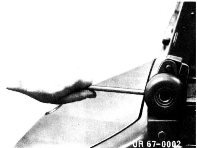
Figure 113 Loosening tensioning screws 404.1
